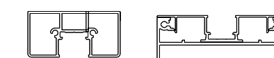
Minimal mullions (i.e., half), 40x80mm and 40x120mm, for framing upon an existing post.
